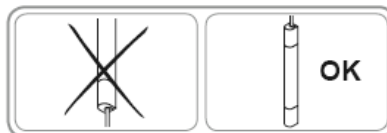
Vertical Battery Tube connector orientation
